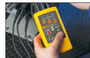
Check the correct rotation of motors prior to connection.
