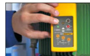
Determine the rotation of running motors by placing the instrument on the motor casing.
