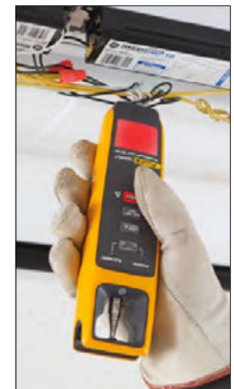
Non-contact voltage: Quickly check for voltage presence
