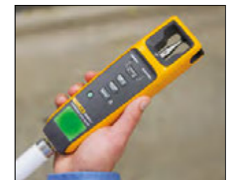
Pin continuity test: Test if filaments have continuity
