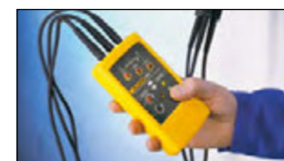
Determine the presence of phase sequence of multiphase electrical supplies.
