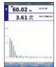
Harmonic spectrum overview with cursors to measure the distortion as a percentage of the fundamental.
