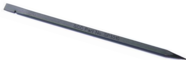
Features pointed tip for holding components whilst soldering, flat end for spudging leads and notch to assist in hooking wires.
