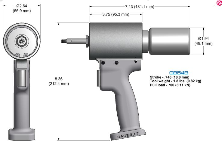
The GB54B pneumatic installation tool is designed specifically for the most efficient installation of blind rivets. GB54B incorporates a collection bottle system to collect spent pintails into a bottle eliminating FOD. It will install aluminum fasteners through 5/32" diameter, and through 1/8" diameter fasteners in any material. It weighs only 1.8 lbs. (0.82 kg) and can operate in any position.
