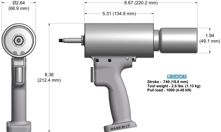
The GB55B pneumatic installation tool is designed specifically for the most efficient installation of blind rivets. GB55B incorporates a collection bottle system to collect spent pintails into a bottle eliminating FOD. It will install aluminum fasteners through 3/16" diameter, and through 1/8" diameter fasteners in any material. It weighs only 2 1/2 lbs. (1.13 kg) and can be operated in any position.
