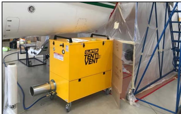
Attach Tent & Vent Filtration System to tent, then add tubing to reroute exhaust if desired.
